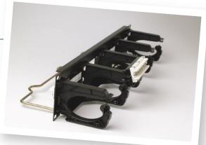
The 19-inch rack mountable patch panel is designed to accept 4 or 8 six-port Distribution Modules (DM) which can be rotated forward, allowing front access to the 110 type IDC terminals for easy cable termination. Built-in horizontal patch cord management brackets provide support for patch cords as well as a holder for the DM modules during installation.
